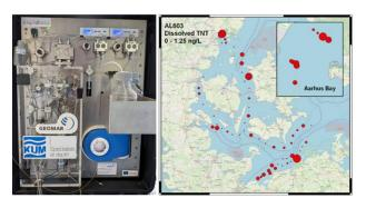
Fig 2. Left panel shows the prototype Xplotector system at sea on AL603. Right panel shows TNT concentrations in deep water along the ship track, measured shipboard with the Xplotector.
