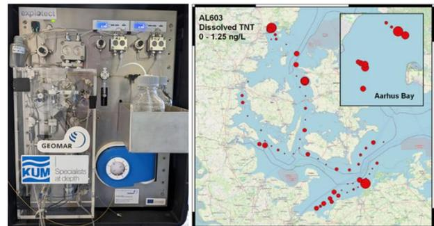
Fig 2. Left panel shows the prototype Xplotector system at sea on AL603. Right panel shows TNT concentrations in deep water along the ship track, measured shipboard with the Xplotector.
